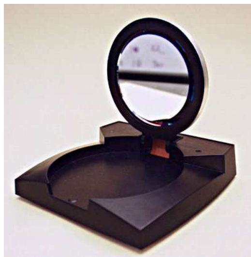
Fig. 2 MONTAGE demonstration camera The folded optic is housed in the upright round disk. Electronics for processing and communications are housed in the platform base.
